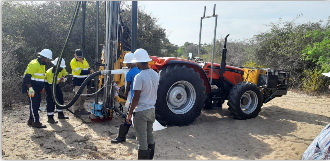
Figure 15 RC aircore tractor mounted drilling rig owned and operated by Titanium Sands Ltd.
