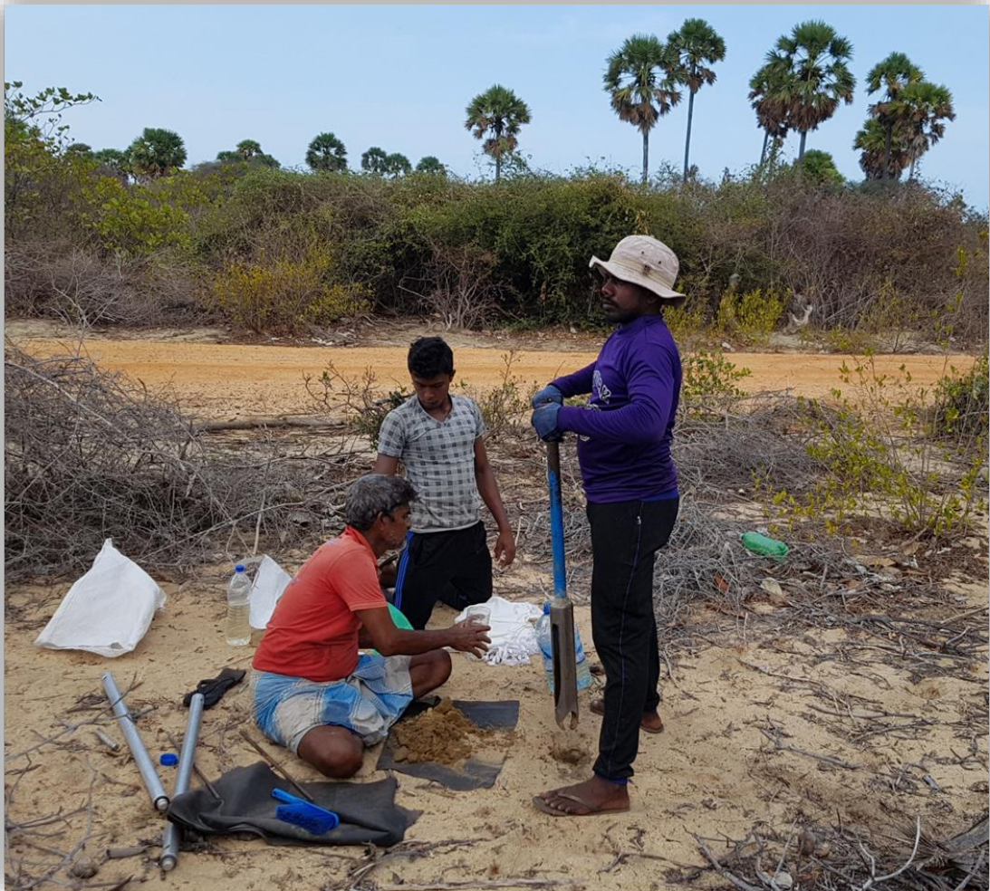
Figure 9 twin hole drilling under supervision by GeoActiv (Pty) Ltd.
