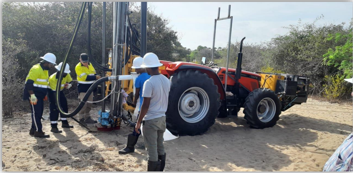
Figure 7 RC aircore tractor mounted drilling rig owned and operated by Titanium Sands Ltd.
