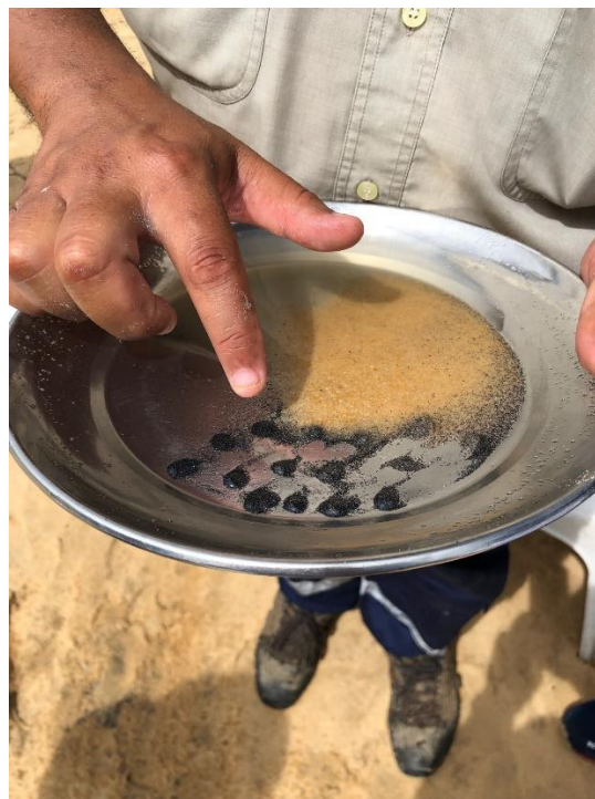
Figure 2 Panning of RC aircore samples from below the water table, during logging at the Mannar Island Project. Dark material is heavy minerals.
