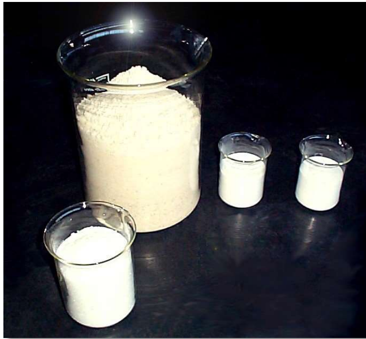
Figure 7: High Purity Alumina produced using the Griffin Process
