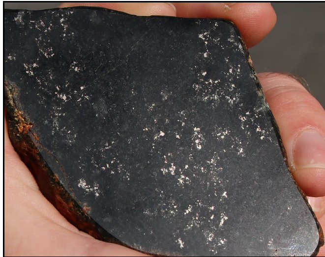
Figure 1. Quick Shears outcropping nickel-copper sulphide hand specimen
