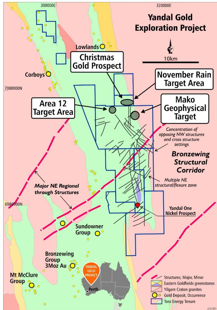
Figure 3: Main focus areas of the first-pass aircore drilling program for the Yandal Gold Project. The map also shows the Interpreted Bronzewing Structural Corridor with main regional structures identified from regional magnetic imagery as well as the main NE structures identified in the large zone of closely spaced NE trending structures and associated fractures within the Yandal Gold Project tenure identified from detailed airborne magnetics and ground gravity geophysical data. State government regional geological mapping has been used for the background geology.
