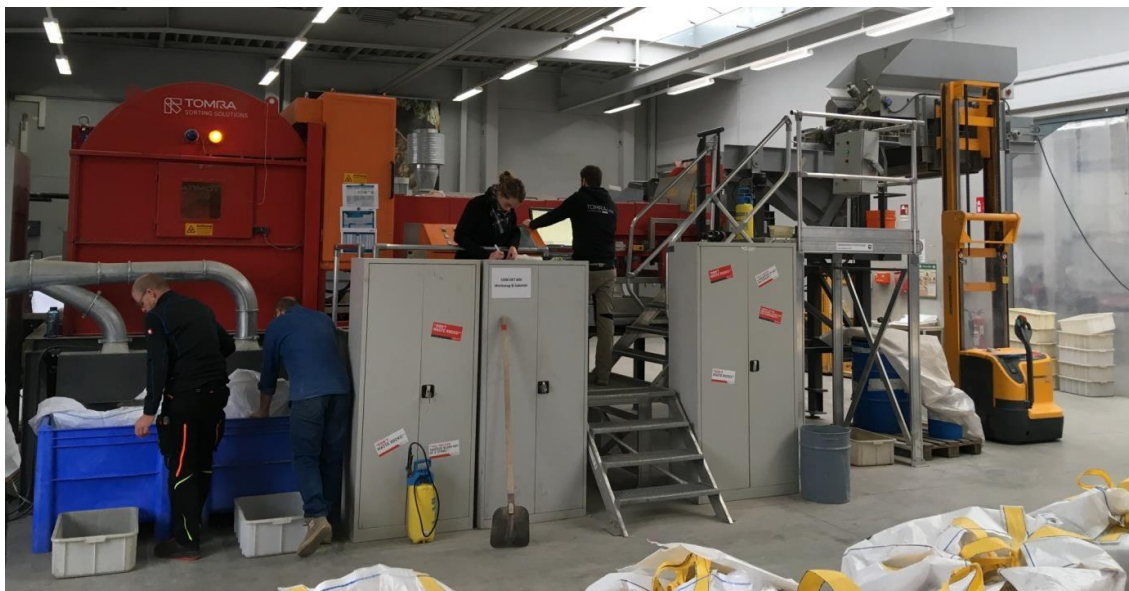
Figure 4: XRT sorter: 3D model of XRT sorter (top) and XRT sorter test rig in Tomra's technical center
