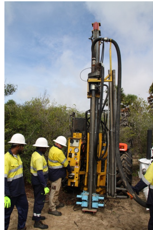
Mannar Island team drilling exploratory RC aircore holes
