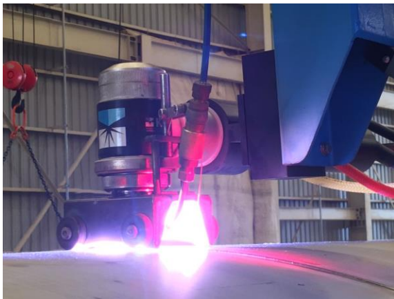
K-TIG's single pass welding of 9mm thick stainless steel
