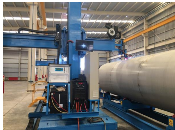
K-TIG circumferential welding system
