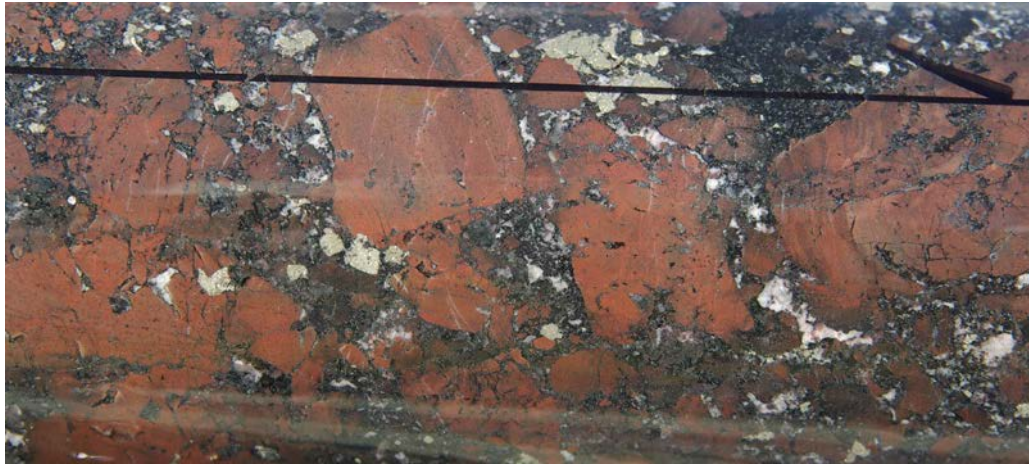
Figure 2 Breccia intersected in Havilah diamond drillhole BADD009 on the eastern side of the Bassanio IOCG target lying within the ML. This hole was drilled in 2016 and intersected potential IOCG host rocks.
