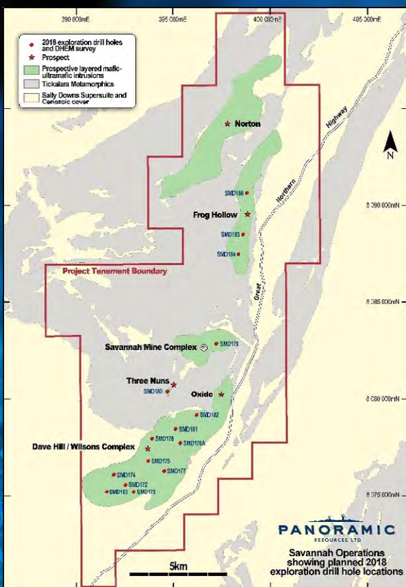
Figure 10 – Savannah Project Plan showing location of prospective mafic-ultramafic intrusions and FY2019 completed drill holes.
