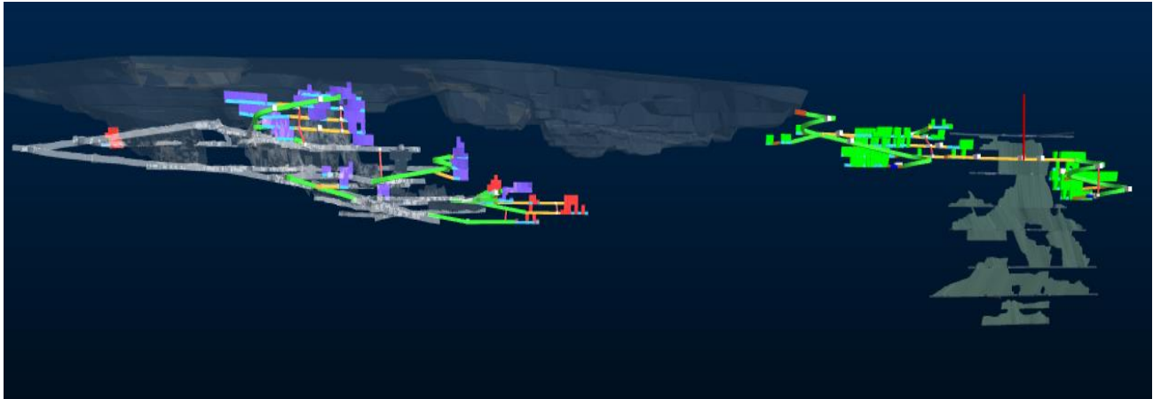
Figure 5 – Long section showing areas identified for mining. Dahmu Lode shown in purple, Hadfield Lode in red and Main Lode in green (north and south of historic stopping shown in grey)
