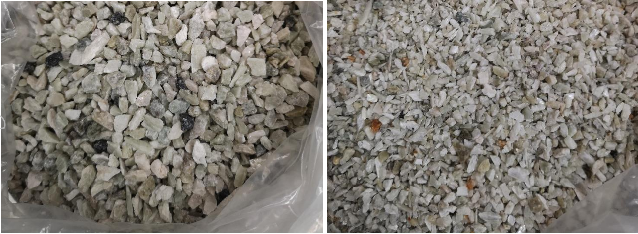
Figure 3. Coarse and fine final DMS concentrates produced from Piedmont composite samples
