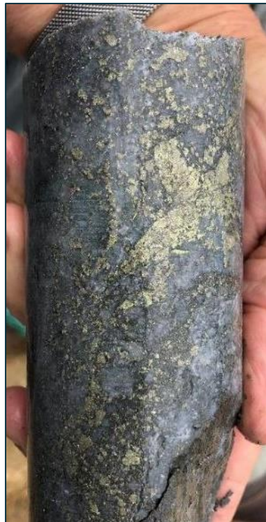
LMDD002, 890.5m, coarse grained chalcopyrite + pyrite
