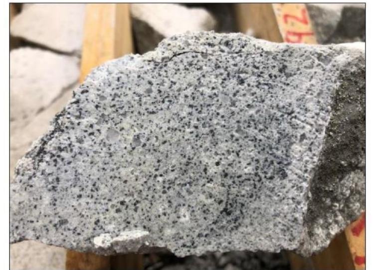
LMDD004 at 68.18m showing black chalcocite and bornite (copper sulphide species) spots through vuggy silica and clay altered volcanic rocks in a 'high sulphidation system'. The interval 68 – 69.6m returned assays of 1.11% copper, 0.2g/t gold, and 5.4g/t silver.
