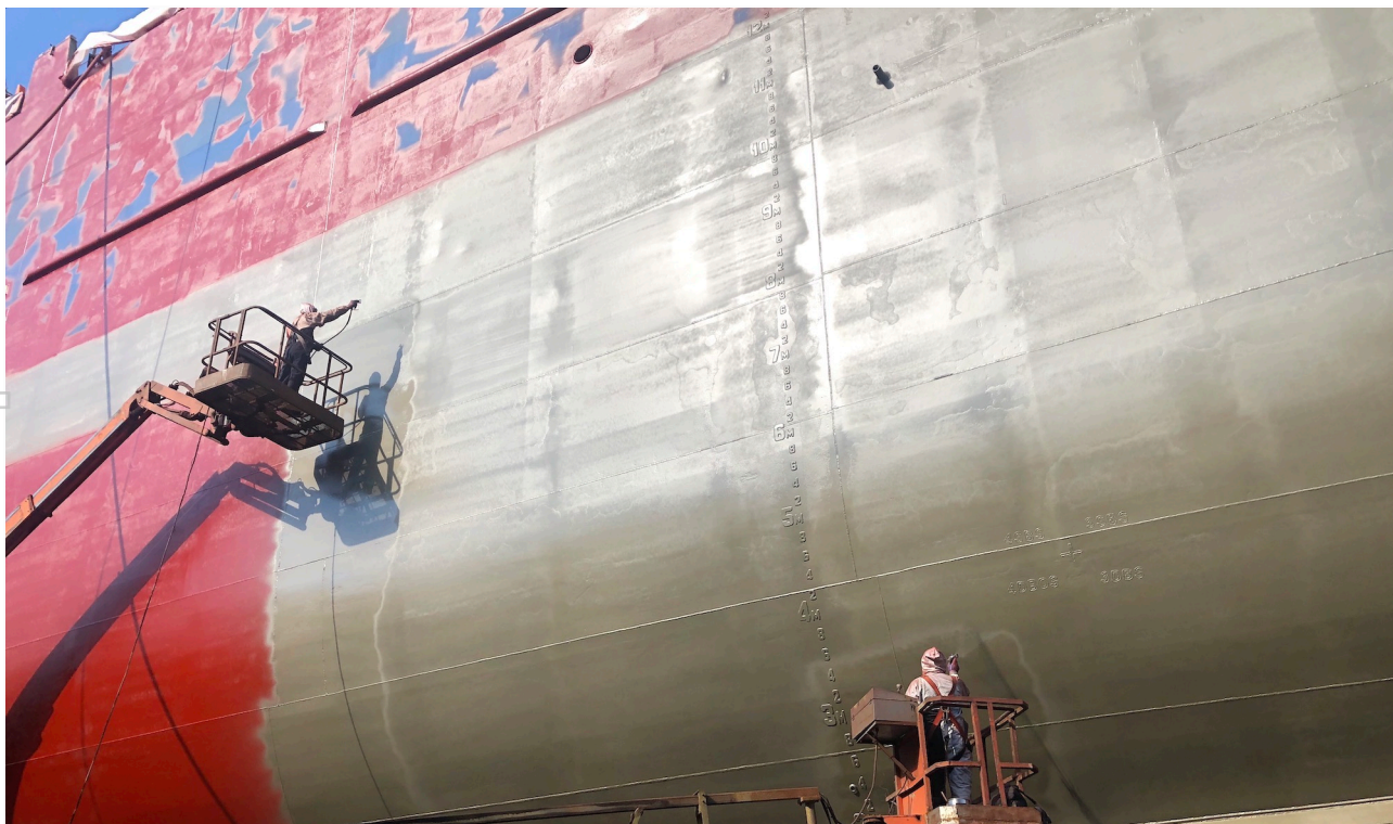
Figure 3 Talphene®-enhanced primer (left) being spray coated onto starboard hull of vessel, alongside the test reference coating (right).
