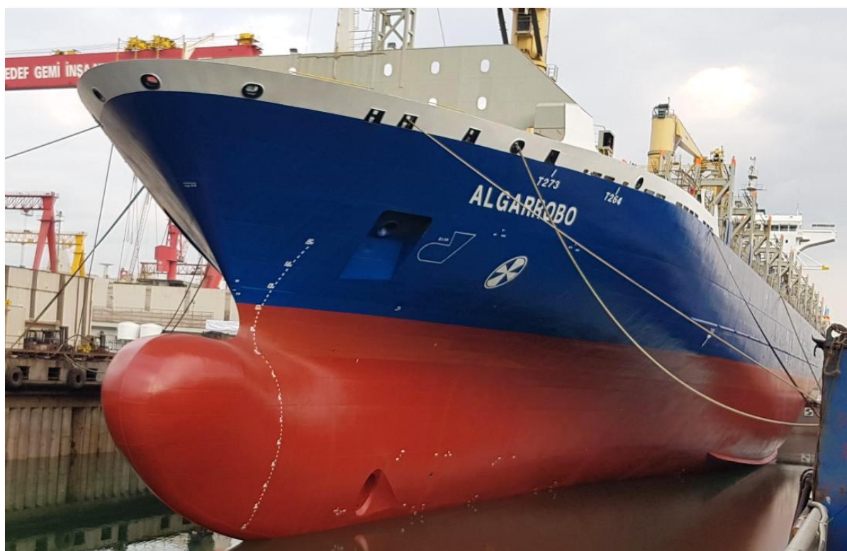
Figure 1 The 33,000 tonne 225m long cargo ship “Algarrobo” leaves dry dock after re-painting including 700m 2 section of Talphen®-enhanced primer coating along the starboard side.
