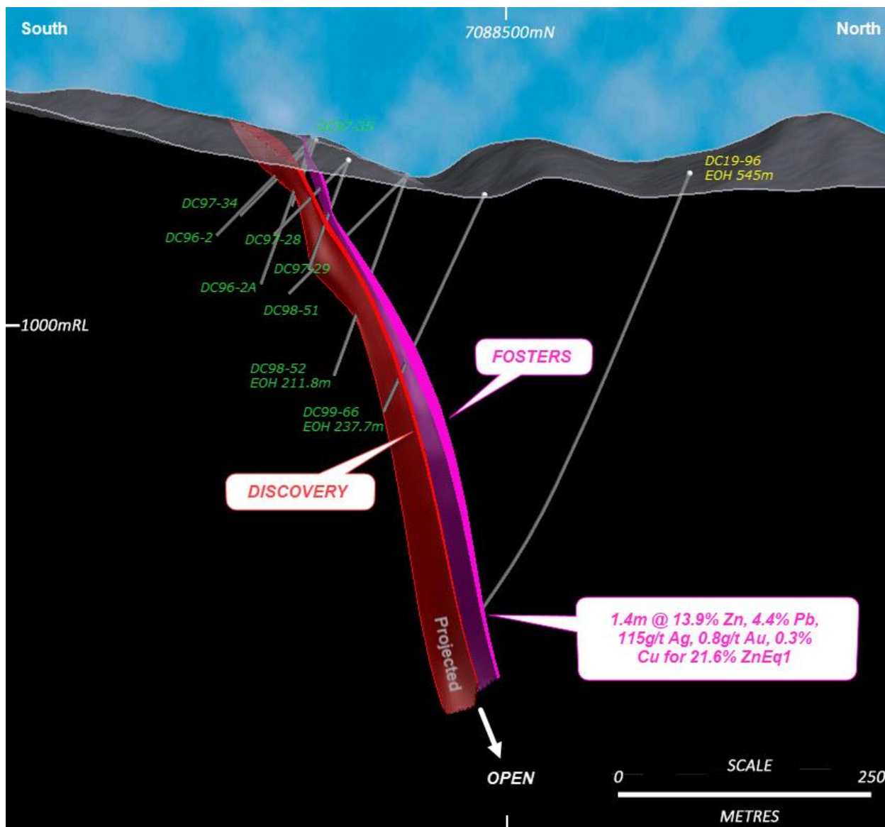
Figure 1: Dry Creek deposit: 3D cross section 480,745mE looking west, with recent drill hole DC19-96 and shallower historic drill holes across a 135m window. The cross section shows the interpreted extension of the Fosters and Discovery lenses with drill hole DC19-96 only intersecting the Fosters lens before being terminated due to poor ground conditions; the Discovery lens remains untested by DC19-96.
