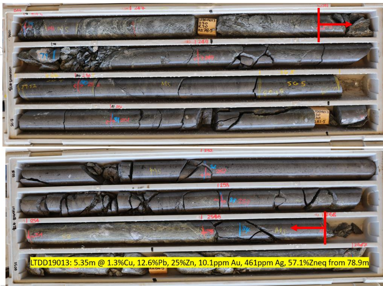
Figure 3 High-grade polymetallic massive sulphide mineralisation with precious metals (LTDD19013, New Queen Lens)
