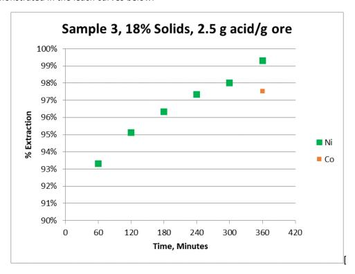
Based on the bench scale testwork, a total acid addition rate (100% equivalent) of 2.5 t/t (dry) ore, a leach temperature of 110°C and residence time of 6 hours were selected for the Ore Processing Plant. Metal extractions assumed for the PFS are provided in the table below:
