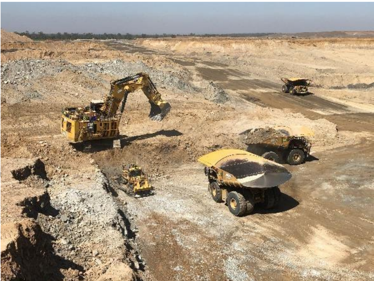
Figure 1: Stanmore's CAT 6060 excavator while commissioning – Pit 2 CDX
