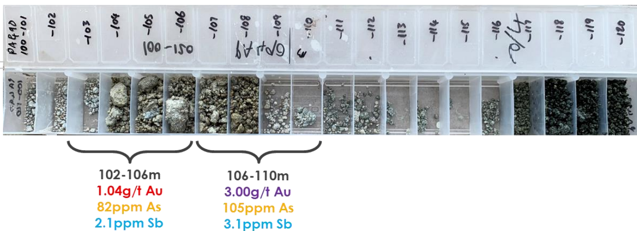
Figure 8. AC drill chips and significant assay results from PA490 – interval from 100m to 120m.
