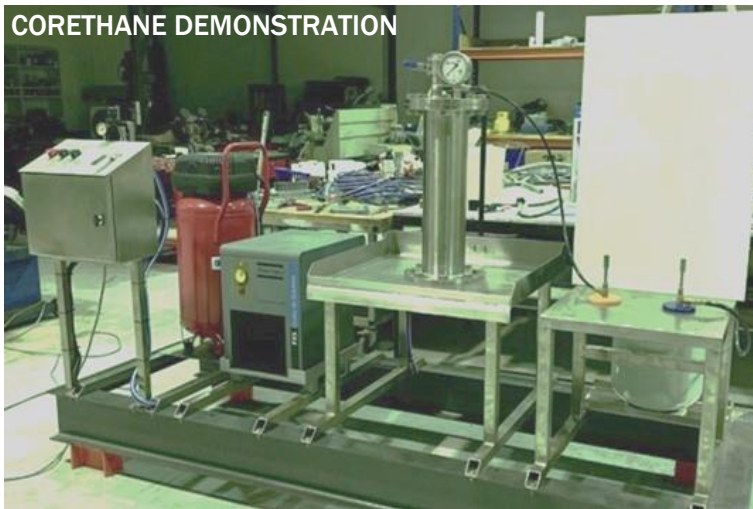
Figure 7: Corethane demonstration unit Alcore refining has reduced the ash content of Hunter Valley coal (Ulan D seam) from 28.5% to 0.3% (see latest ABx Quarterly Report). Alcore engineers have constructed a Corethane combustion demonstration unit to compare gas and Corethane by burning in two Bunsen Burners, one burning LPG gas and the other burning Corethane so as to compare the two flames against the white background panel. It shows that both flames equally emit zero soot, smoke or un-burnt particulates. The main difference is the cost – Corethane costs are much lower than the cost of gas.
