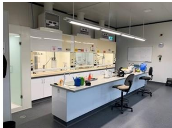
Figure 4: ALCORE test lab, fume cabinets with hi-tech scrubbers, showers, microscopes & Draeger air monitor (wall)
