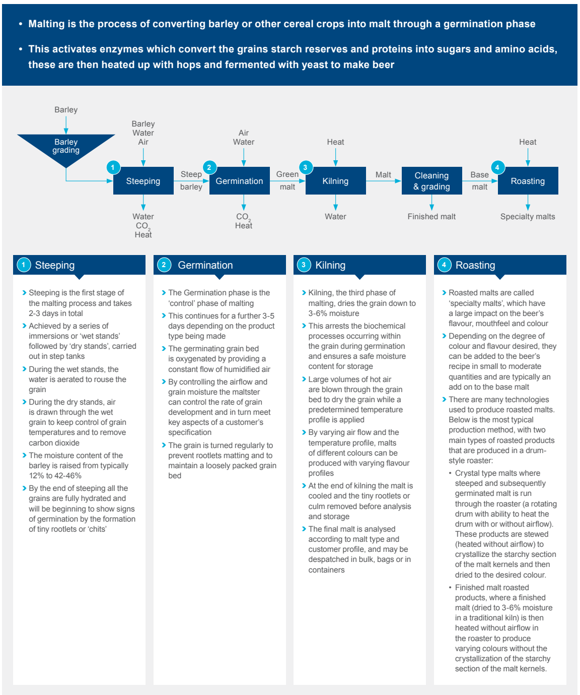
Figure 2.3(a): Overview of the malting process
