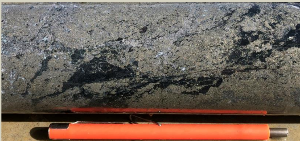
Massive pyrite+low-iron sphalerite. High-grade Zn interval. 361.0m
