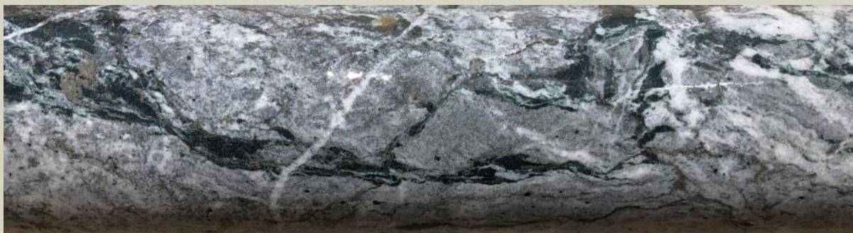
Intense pervasive dolomite+calcite+quartz-altered microdiorite with refolded shear fabric cut by late quartz+carbonate stringer veins. 260.7m
