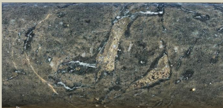
Microdiorite. Moderate pervasive chlorite+carbonate±biotite. 5% disseminated and patchy pyrite. 336.8m
