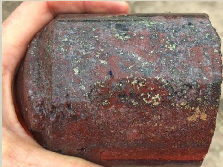
Disseminated chalcopyrite in quartz+hematite rock. 223.4m.
