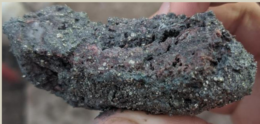
Vuggy quartz, hematite, pyrite and chalcopyrite zone in the UCF at 177.4m
