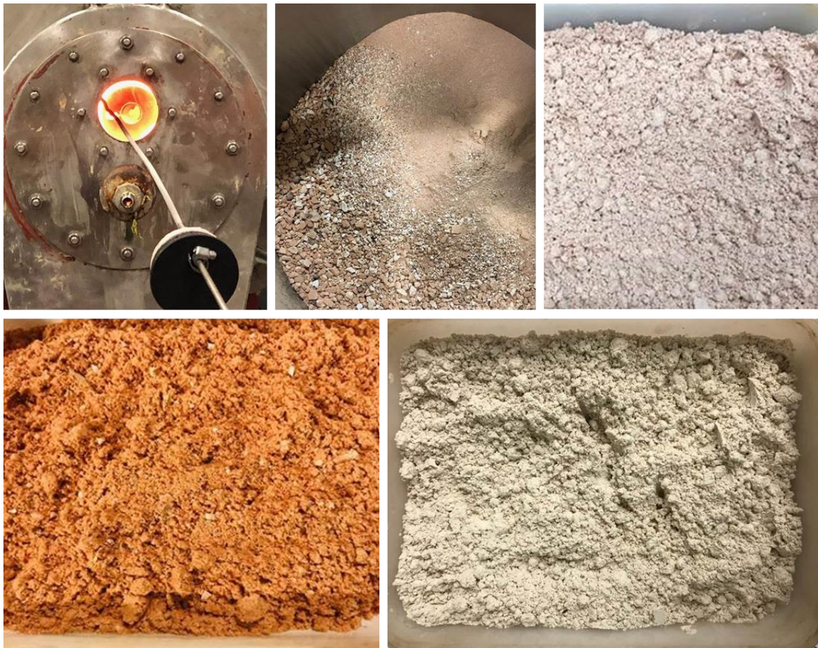
Figure 1 – Spodumene calcination and roasting (from left to right) – (top) pilot kiln, calcined product, milled beta spodumene (bottom) beta spodumene after mixing, beta spodumene after roasting
