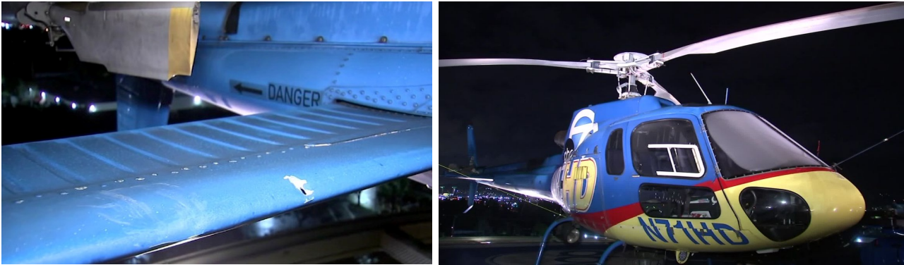
The LA News Helicopter that was struck by a drone at 1,100 ft AGL. The closeup image shows puncture damage to the wing caused by the collision
