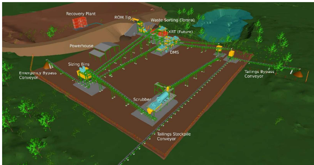
Figure 4: 100tph Plant Design
