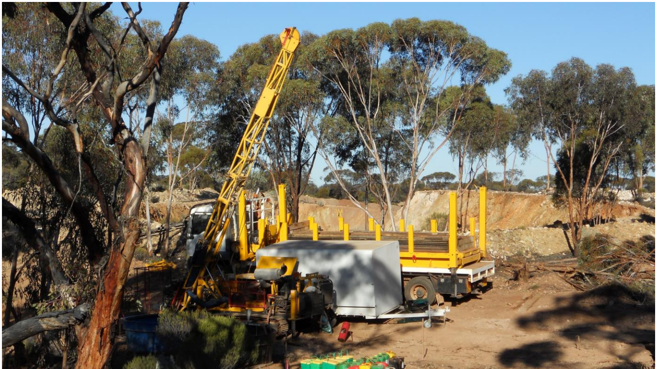
Figure 5. Topdrive Drilling Australia track-mounted diamond core rig setup and drilling at Munda Gold Project, Widgiemooltha WA.
