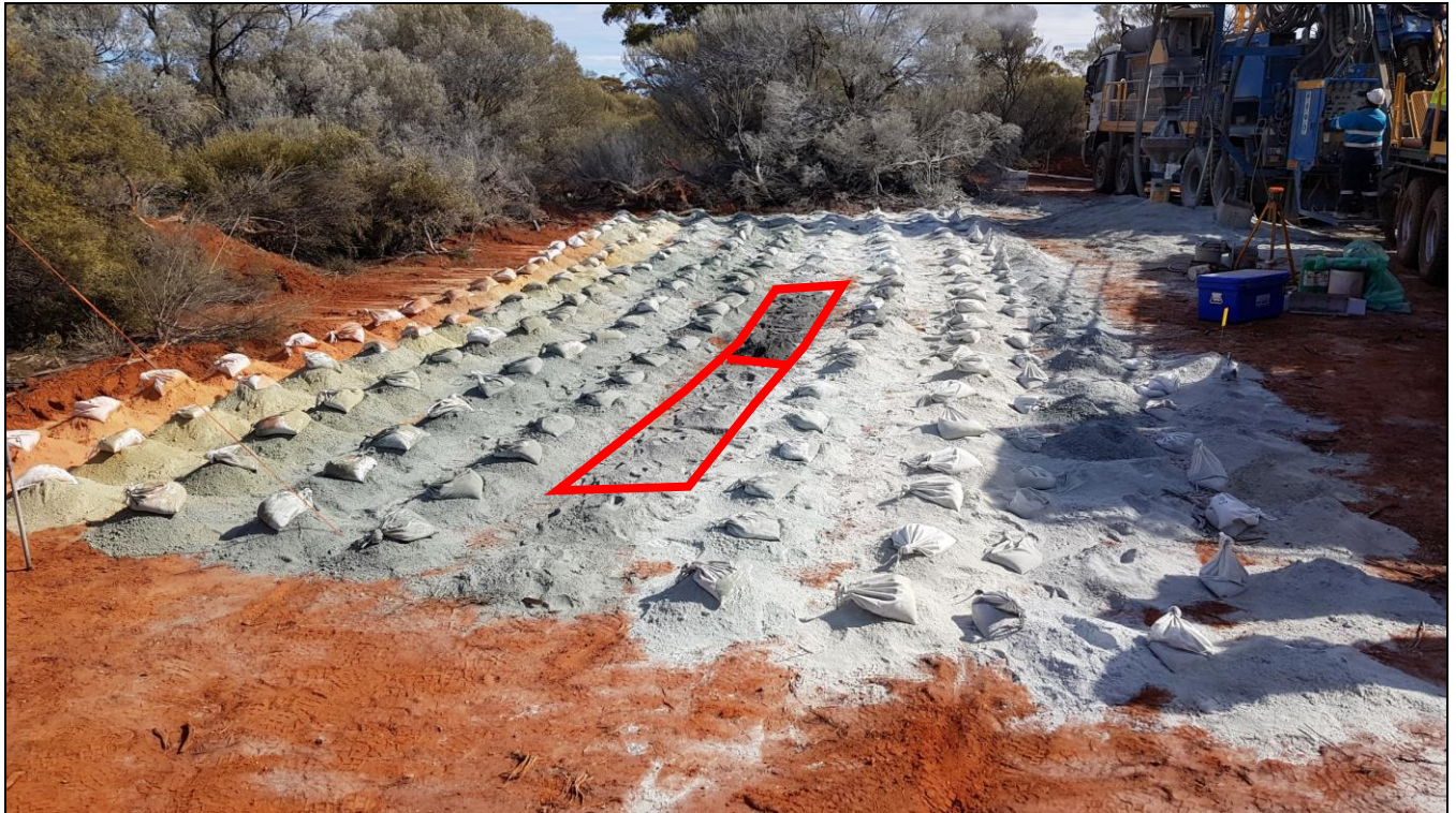
Figure 1. Sulphide mineralised samples within CBP042 at Carr Boyd. Black samples are the higher grade, sulphide rich matrix zone.
