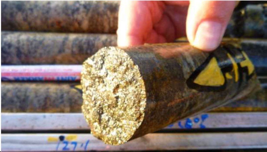
Figure 4: An example of the strongly pyritic (potentially cobaltiferous) bands in albitic gneiss in DD95STV3.
