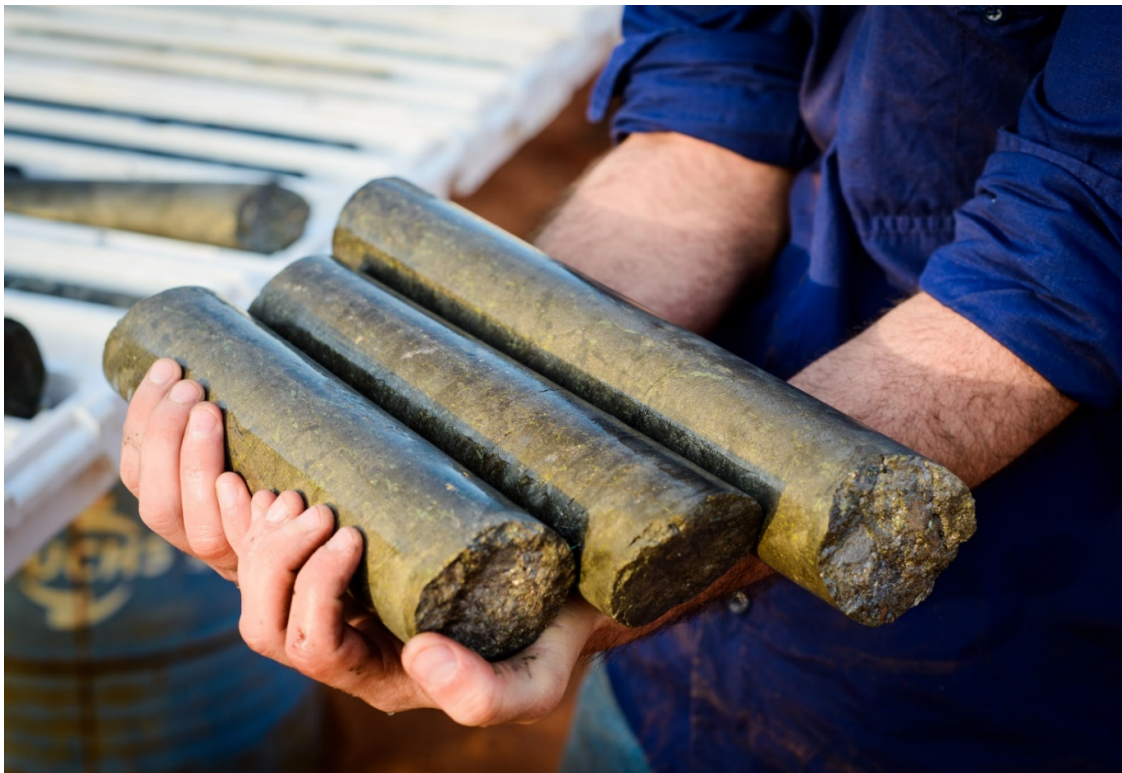
Figure 1 – drill core from MAD152 with massive sulphides that returned assays of 4.29% Ni, 1.46% Cu and 3g/t PGEs from 49.05m
