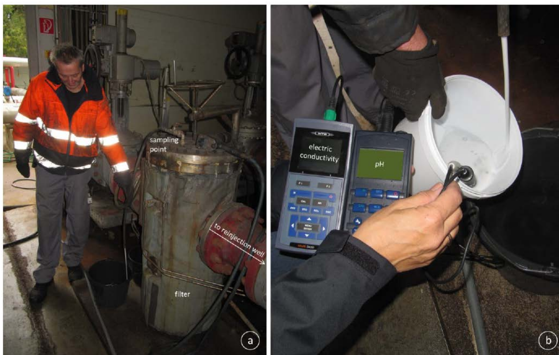
Figure 3: Confirmatory sampling of wells in Upper Rhine Valley by Vulcan team, and measurement of on-site brine parameters.
