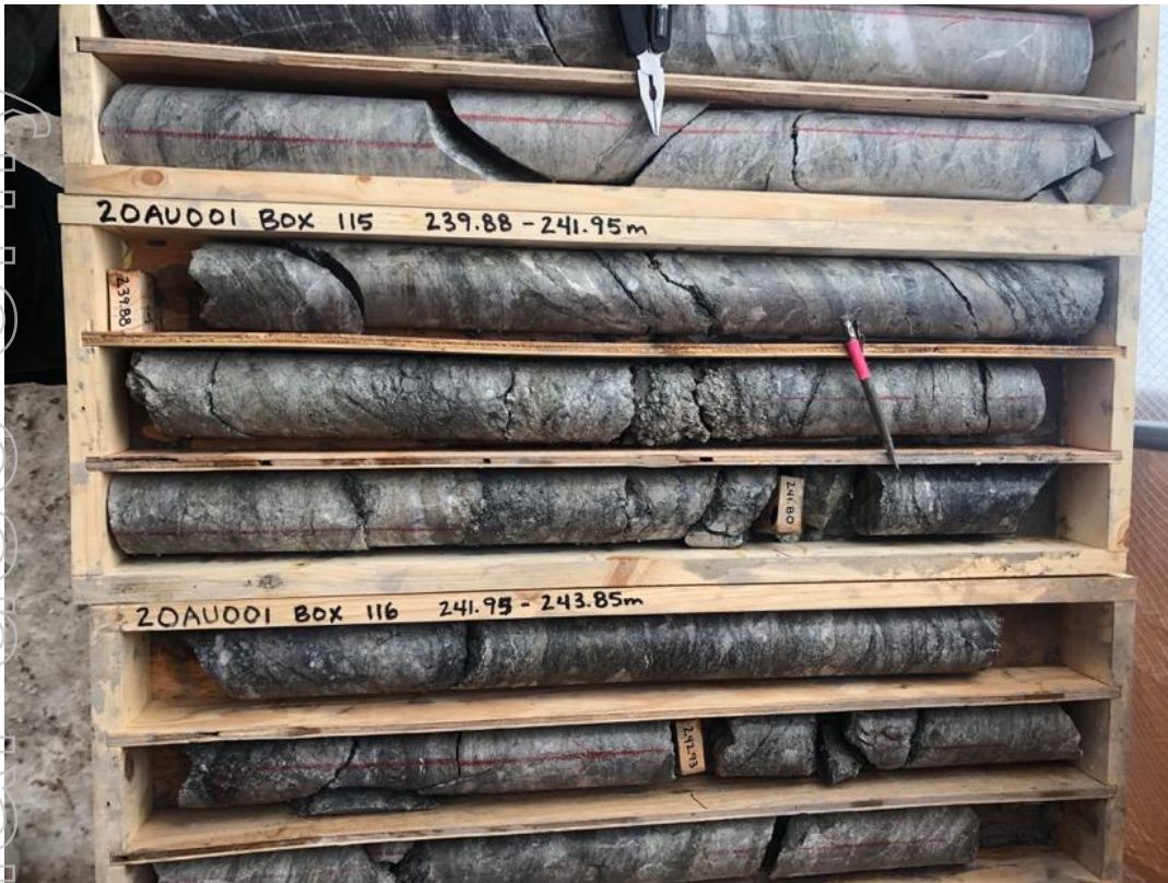
Figure 3. Hole ID 20AU001 box 115 and 116; 239.88m to 243.85m zone(s) of quartz veining with pyrite and arsenopyrite mineralisation in paragneiss.
