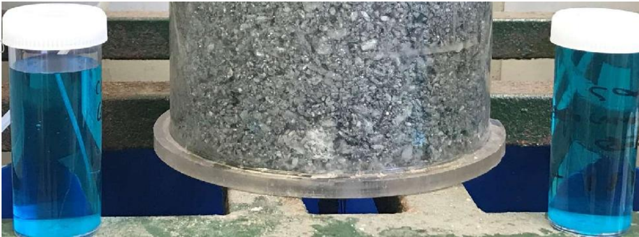
Image 2 / Metallurgical column test-work
