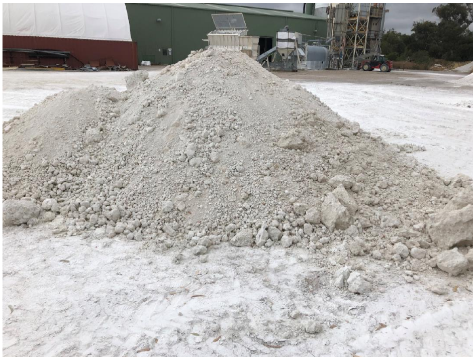
Figure 3 – Carey's Well raw kaolinized granite, after auger sampling. The visible intact lumps are easily broken by hand.
