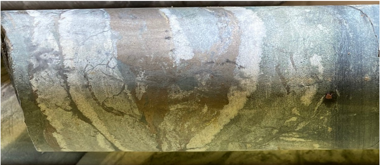
Figure 5: 15cm interval from 20LCDD001 with quartz-carbonate-pyrrhotite vein with carbonate-chlorite alteration selvage overprinting calc-silicate proto banded iron formation.
