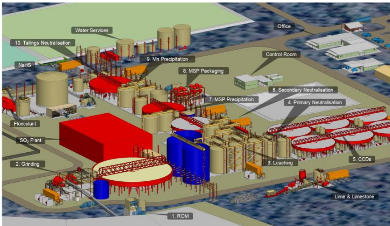
Figure 3 - 3D isometric of the Mt Thirsty processing plant showing generalised process flow (numbered labels)
