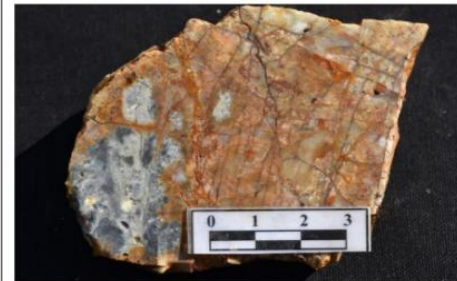
Hydraulic quartz vein and rhyolite host rock breccia, pervasively flooded by mesocrystalline quartz and fine-grained pyrite. Highly oxidised with ubiquitous limonite after pyrite.
