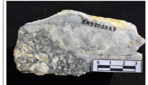
Polyphased hydraulic vein breccia with rip-up vein fragments and a central black sulfidic band comprised of fine-grained pyrite & sulfosalts.
