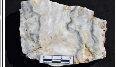
Polyphased hydraulic vein breccia & colloform-banded vein comprised of white mesocrystalline quartz with grey-black sulfidic inter-bands and wispy fills.
