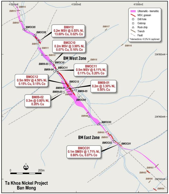
Figure 6: Ban Mong MSV target showing historical trenching and drilling by previous owners (see ASX Announcement 8 May 2019).
