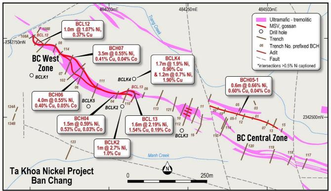
Figure 4: Ban Chang MSV target showing historical drilling and trenching by previous owners (see ASX Announcement 8 May 2019).
