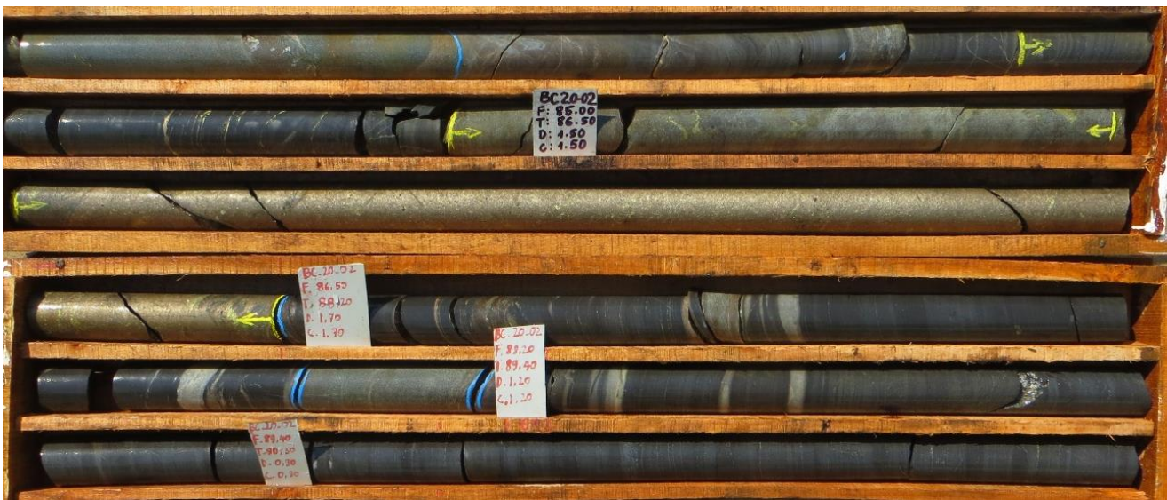
Figure 4: Blackstone's maiden Ban Chang drillhole BC20-02 intersects 1.2m MSV from 87.0m
