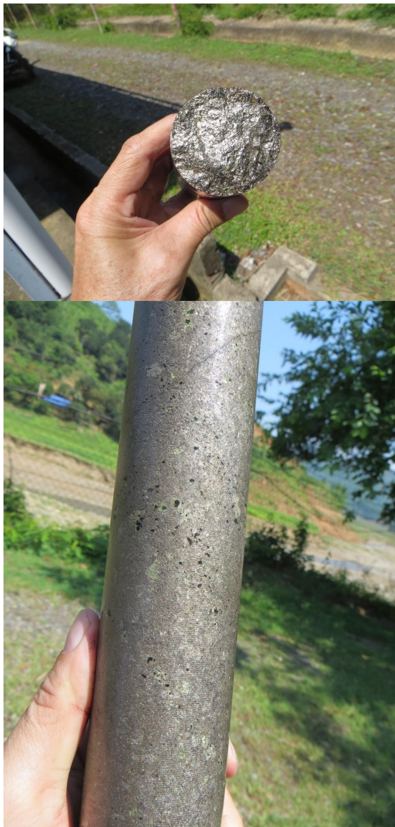
Figure 2: Blackstone's maiden Ban Chang drillhole BC20-02 intersects massive sulfide
