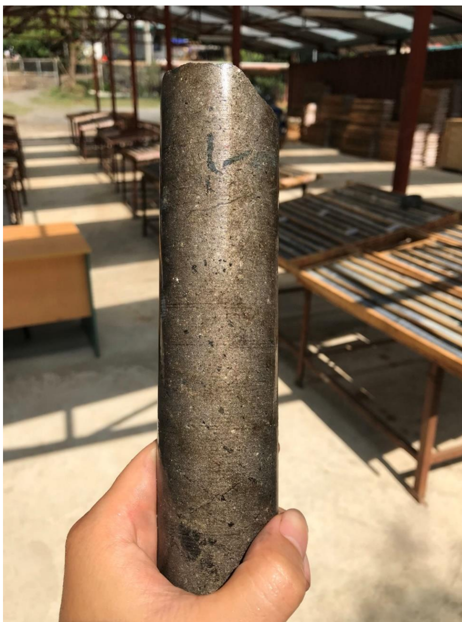
Figure 1: Blackstone's maiden Ban Chang drillhole BC20-01 intersects massive sulfide
