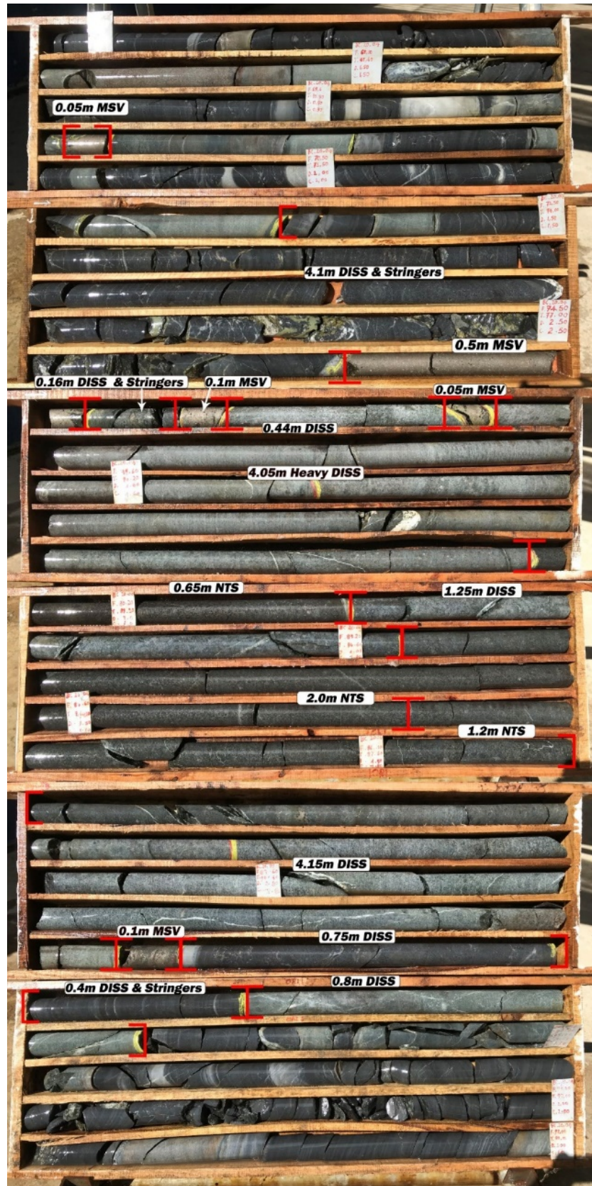
Figure 5: Blackstone's Ban Chang drillhole BC20-04 intersects a zone of 15.4m wide veins of sulfide mineralisation
