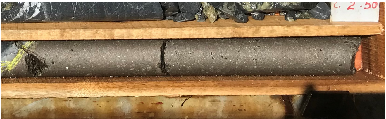
Figure 2: Blackstone's Ban Chang drillhole BC20-04 intersects more massive sulfide
