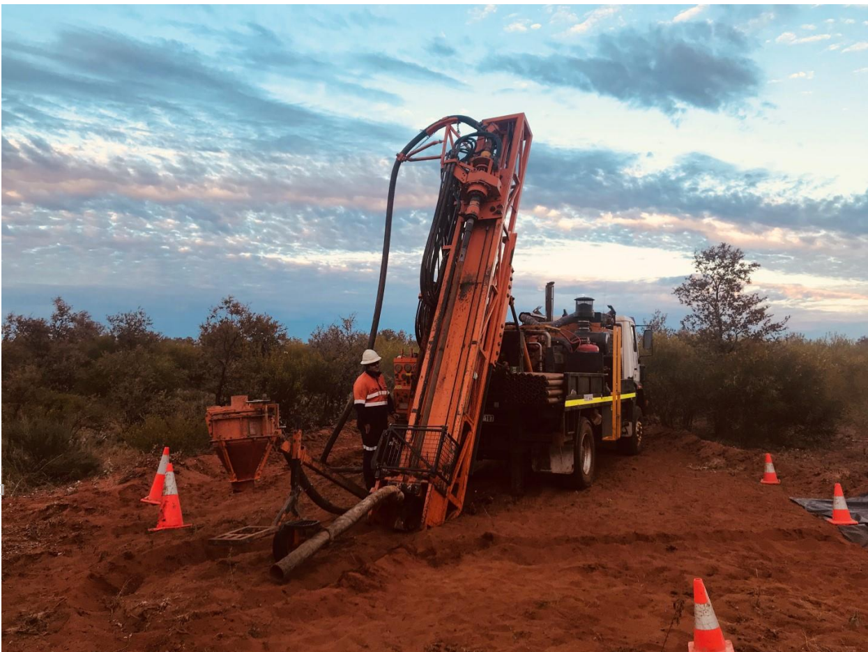
Figure 1: Bostech aircore drill rig on target 1 at the Yule South Project in the Mallina Basin.
