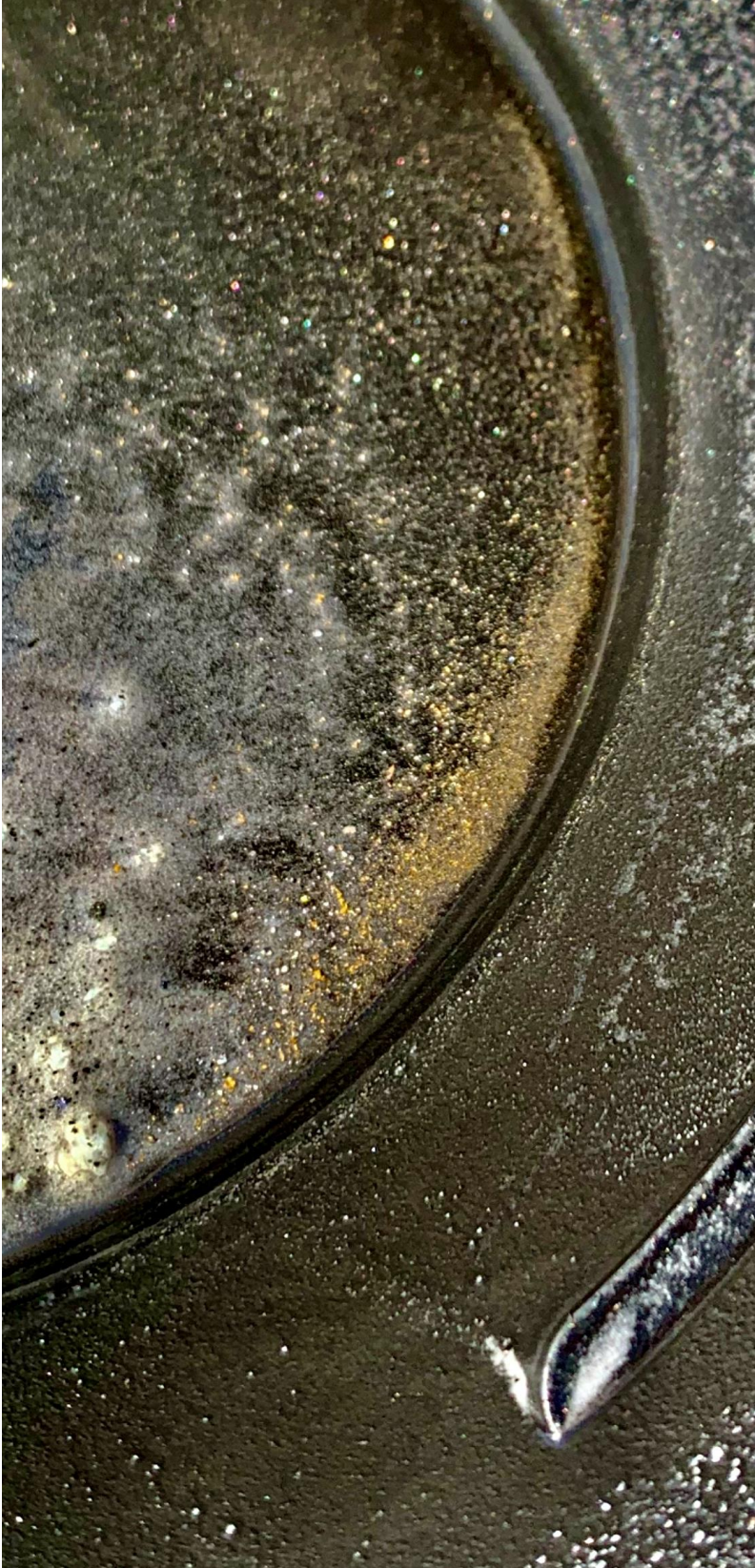
Figure 2: Visible gold in panning dish from hole FKGRC184 at 82-83m grading 304 g/t Au.
