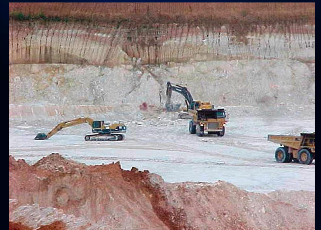
Typical Kaolin Mine with Very Simple, Shallow, Quarry-like Operation
