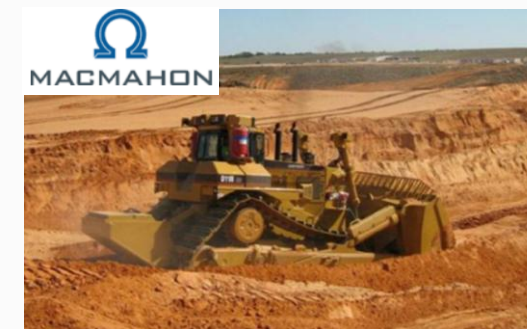
Image: Conventional dozer push mining operation
