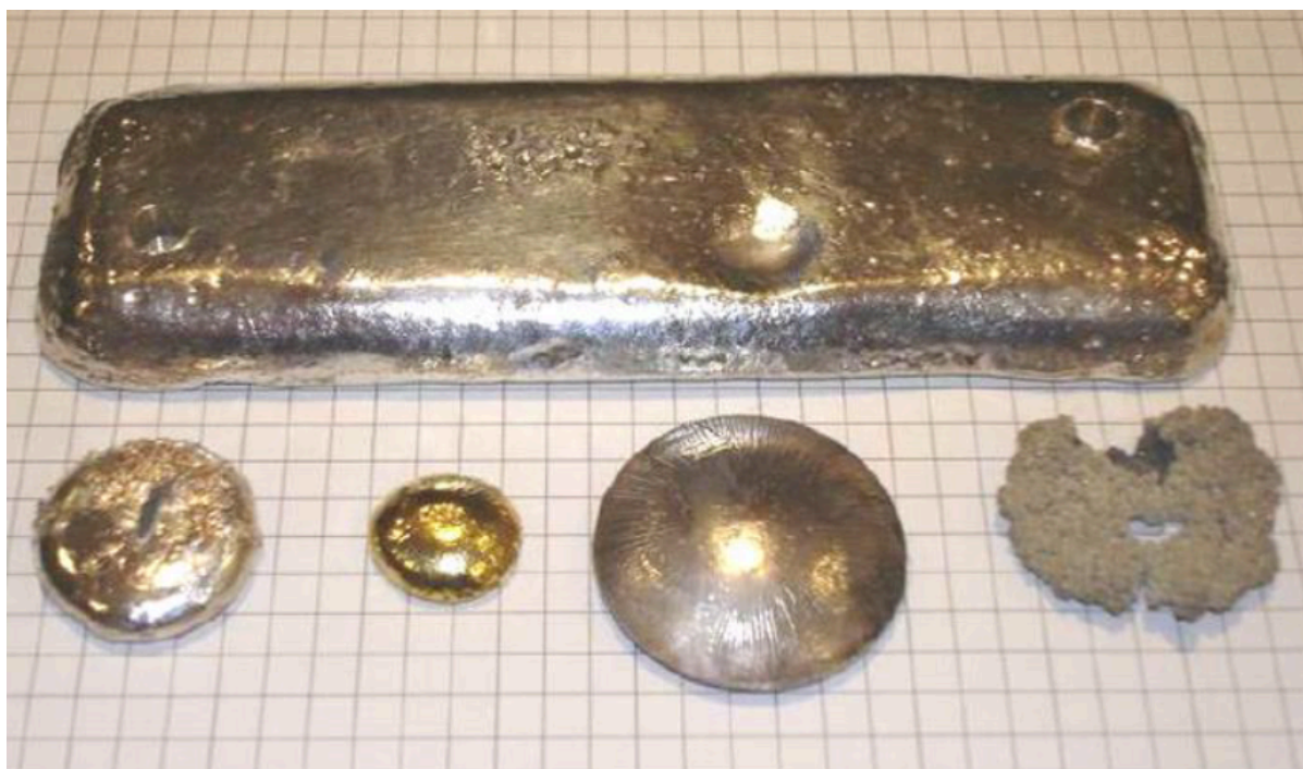
Figure Four – Gold and Silver Dore Produced from the 16.2 Ton Bulk Test
