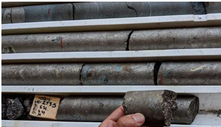
Figure One | Massive Sulfides in TOR05 from drilling at the Thor Prospect
