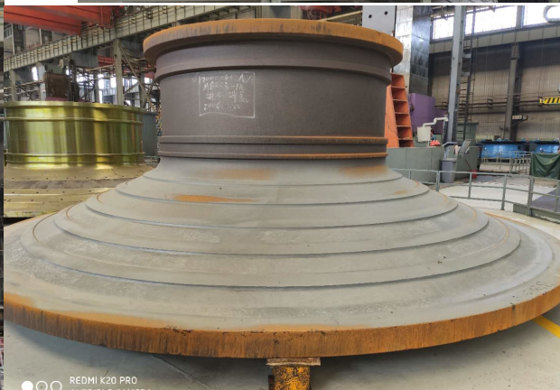
Ball mill head and girth gear manufacture
