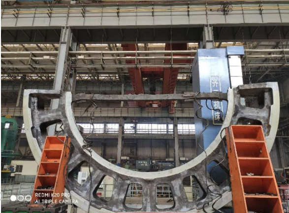
Ball mill head and girth gear manufacture
