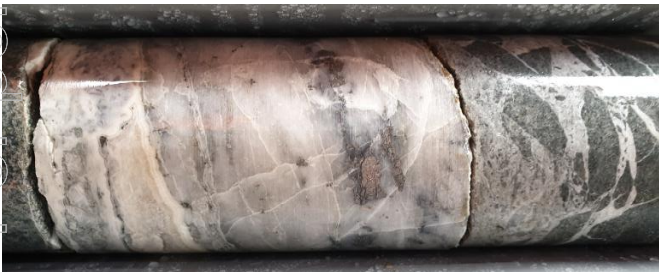
Figure 6. Laminated and brecciated quartz-arsenopyrite vein in diorite within 0.4m @ 2.68g/t Au from 162m in PHD008 – Ironbark South Prospect (drill core is ~63mm in diameter)
