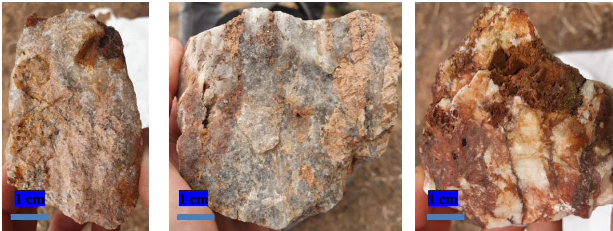
Figure 8. Gradation of veins from K-feldspar dominant (left photo) to quartz-dominant (right photo) with increasing boxwork gossan (dark brown colour) from weathered sulphides.
