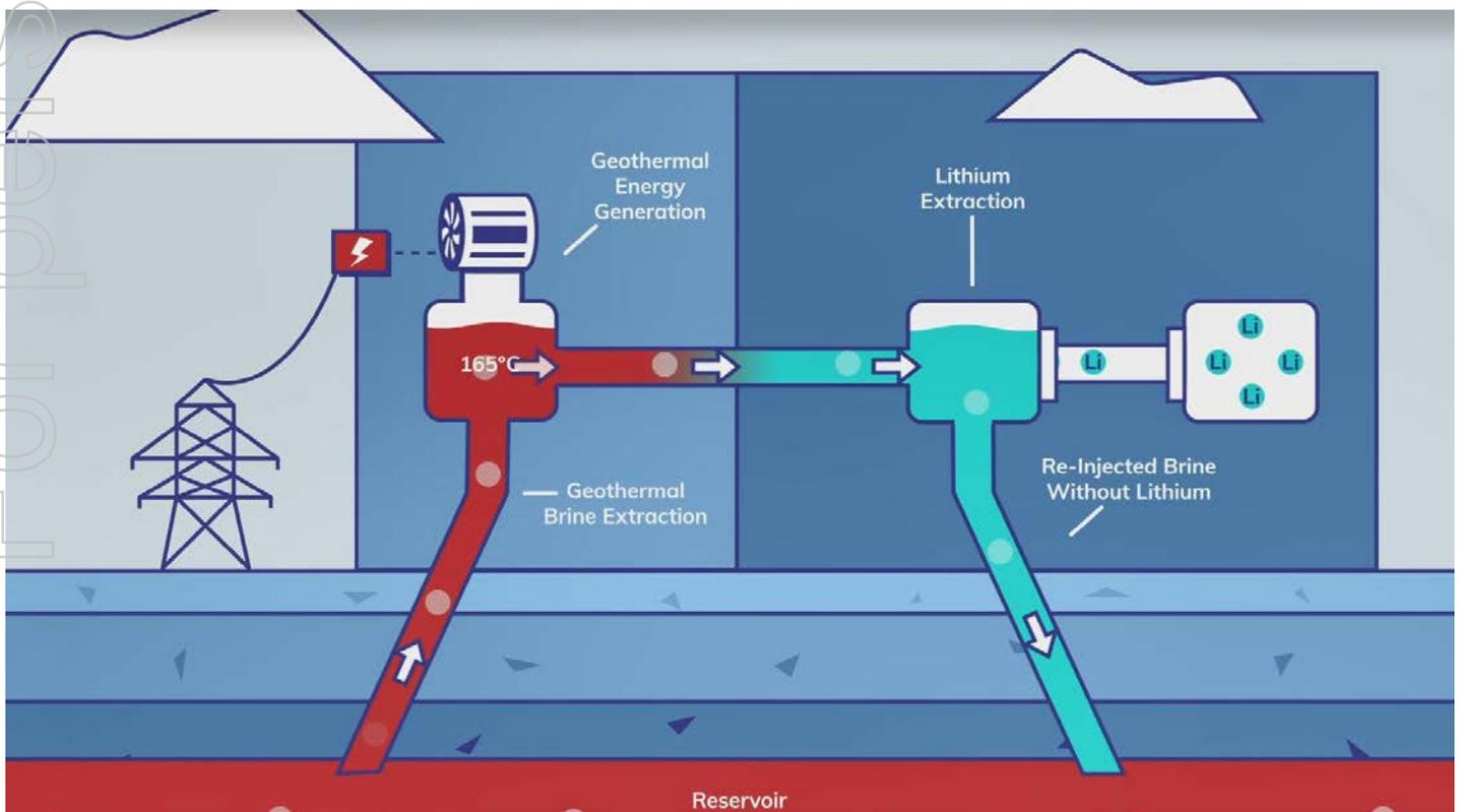
Vulcan is pleased to announce that it has successfully completed initial bench-scale test work on Upper Rhine Valley geothermal brine, using adsorbent-type direct lithium extraction (DLE) technological approaches. Vulcan was able to quickly identify and test the best DLE technology options for the Upper Rhine Valley brine by leveraging the experiences of its in-house team and external consultants, who have worked on multiple geothermal lithium projects with numerous DLE technologies.
