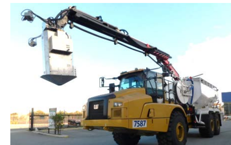
Robotic explosive placement
