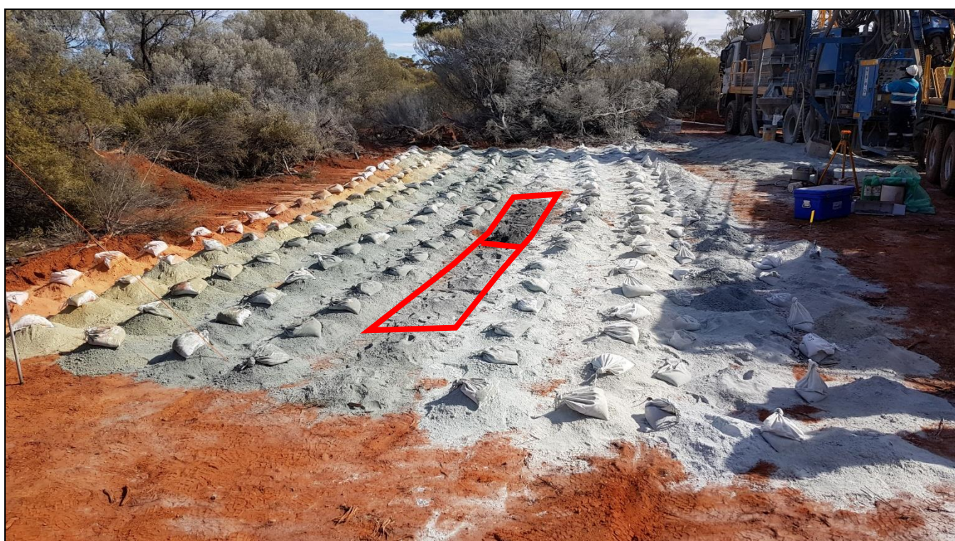
Figure 1. Sulphide mineralised samples within CBP042 at Carr Boyd. Black samples are the higher grade, sulphide rich matrix zone.
